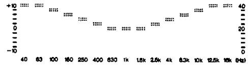
Example: In case the high-frequency range and the low-frequency range are boosted.
